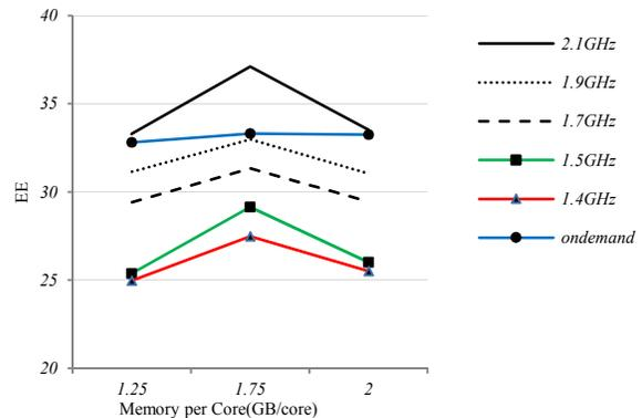
Fig.18. Energy efficiency with different memory per core and CPU Frequency on #1 server.
