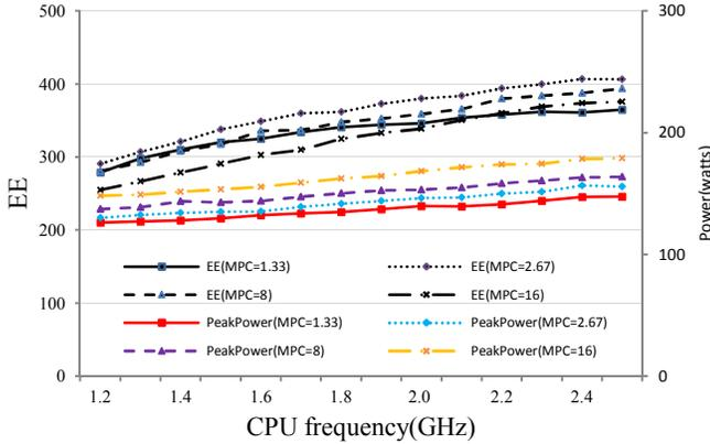
Fig.21. Energy efficiency and peak power on server#4 with different memory per core and frequencies.
