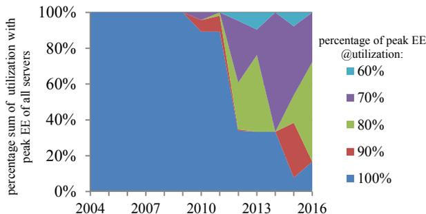
Fig.16. Chronical shifting of utilization with peak energy efficiency.
